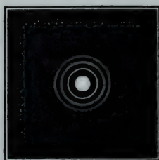
Object-glass properly adjusted.
